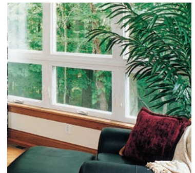
Picture Window over Awning Window
